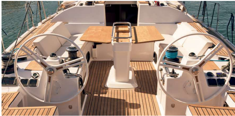
All sheets are running back to the helmsman's steering position, making sail trimming simple and accessible.
